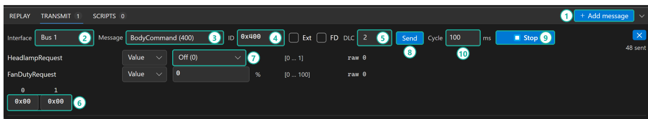
Figure 36. Sending a message defined in the DBC file
