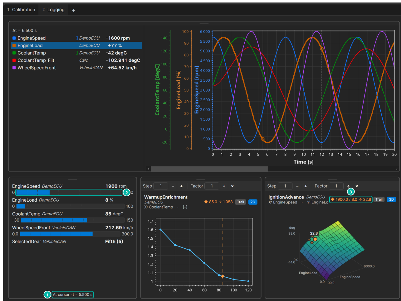
Figure 15. Analysing a recording: a plot across two devices, with readouts, bars and working points at the cursor
